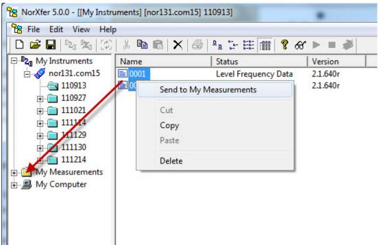
After transfer to PC, the files can either be converted to Excel using the "Convert To Excel" or the "Overview (Excel)" functions
