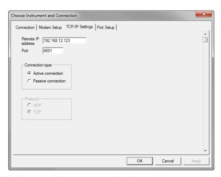
Port: IP port number (set up on modem, eg. 4001 on Moxa)
