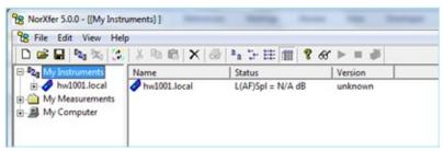
Mark the measurement files that you want to copy onto the PC. Use drag and drop to the "My measurements" catalogue or right click and select "send to My Measurements"
