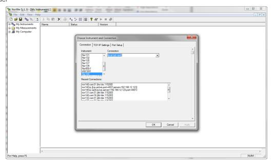
Mark the measurement files that you want to copy onto the PC. Use drag and drop to the "My measurements" folder or right click and select "send to My Measurements"
