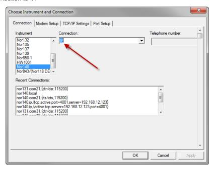
Remote IP address: IP address or name of remote modem
