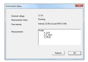
The status info includes battery voltage, memory left and which parameters are measured:
