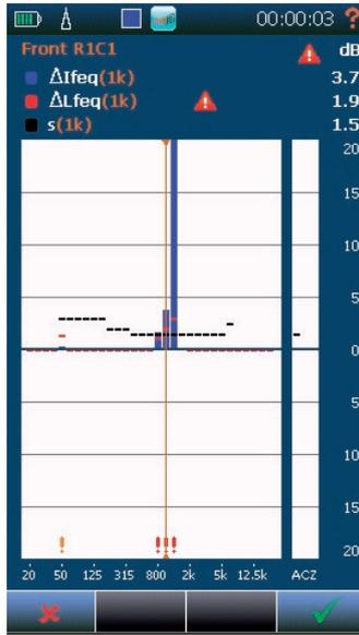
The Δ-view shows the difference between two orthogonal scans
