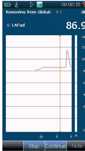
The Pause display allows a chosen number of seconds to be removed from the measurement
