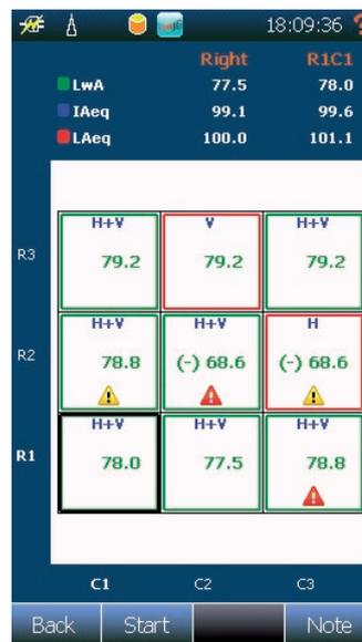
Several segments in a surface. Warnings indicate problems, borders indicate if the segment is completely measured or excluded
